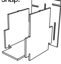
Insert one SIDE PANEL into the BACK vertical slot. Repeat with the other side panel. Insert the SHORT extension of the BOTTOM PANEL into the back horizontal slot.
