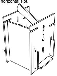
Place one notch of the small RECTANGLE (long edge up) into the BACK slot. Slide down the FRONT panel until it slips into the slot.
