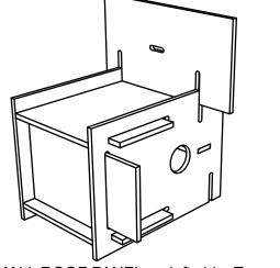
Slide the SMALL ROOF PANEL on left side. Turn the birdhouse on its side to push until the notch snaps. Slide the LARGE ROOF on the right side.
